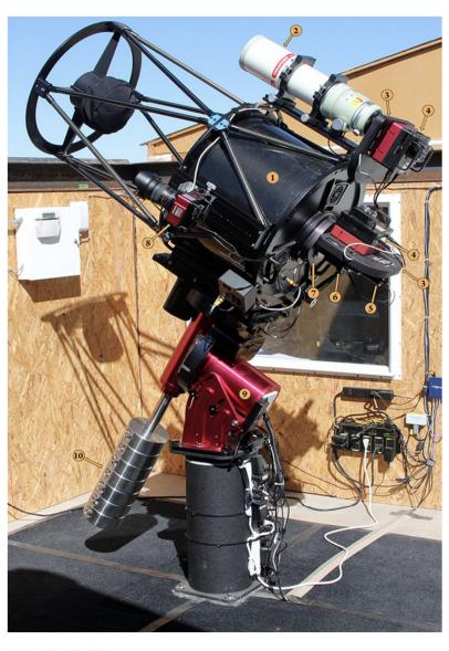
PlaneWave 20-inch 1/6.8 CDK Telescope Takahashi FSQ-106EDX3 Apochromatic Refractor SBIG FW7-STX Filter Wheels (2) SBIG FW7-STX Filter Wheels (2) SBIG STX-16803 Monochrome CCD Cameras (2) Starlight Xpress Lodestar X2 Autoguider Innovations Foresight 10n-Axis Guider XM Finger Lakes Instruments Atlas Digital Focuser SBIG STF-3300 CCD Camera w/ Rokinon 16mm Lens Paramount ME II German Equatorial Mount Stainless Steel Counterweights (5) SBIG SAIISAY-340C Camera
